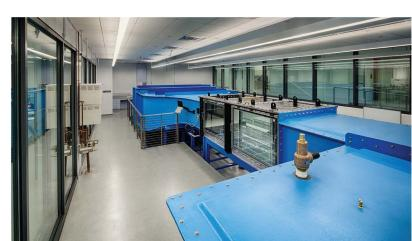
The Hydrology Lab water tunnel operates at 0.15 m/s (0.49 fps) to 1.50 m/s (4.92 fps)
